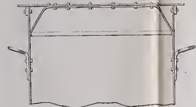
SECTION SHEWING THE LID IN POSITION. BIRMINGHAM PAIL AND COVER. Scale 1/2 Inch = 1 Foot
